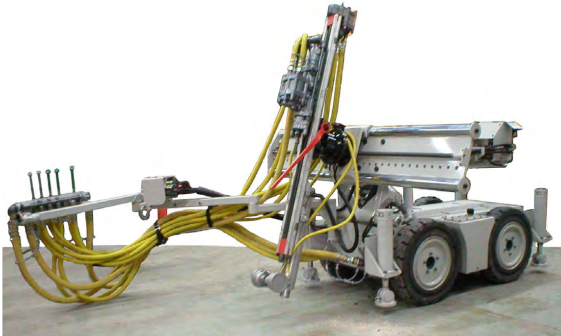
PHQ36IR Long-Hole Drill Set-up on a PHQ3000LHP Pneumatic Carrier
